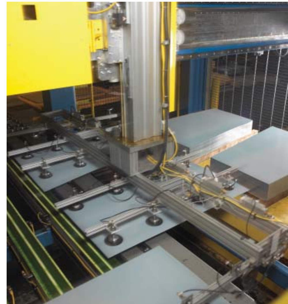
Suction cups enable stacking of ferrous or nonferrous blanks. Seen here is a double-blank stacking operation, where blanks produced by the oscillating shear are stacked neatly. Towmotors then route the stacks to one of three blanking presses.
